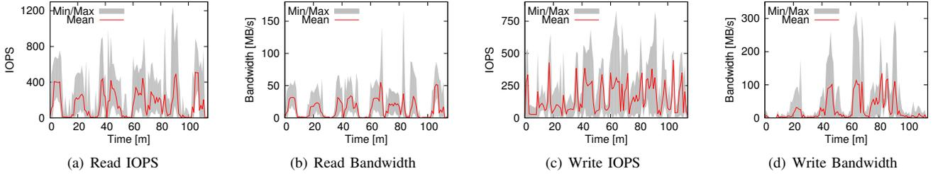
Fig. 5: I/O utilization of the cluster sampled every second and aggregated per minute during the execution of the BTWorld workflow on the 10 GB data set. The gray areas represent the range of observed values.
